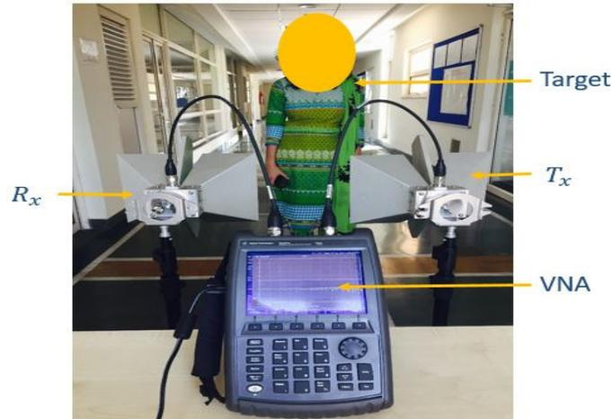
Figure 4.5: Monostatic CW radar configured using a vector network analyzer and two linearly polarized horn antennas for five distinct carrier frequencies - 2.4, 3, 4, 4.5 and 5.8GHz
