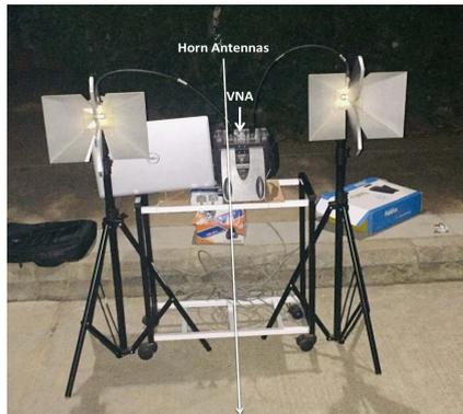
FIGURE 3.1: Monostatic radar configuration using vector network analyzer in narrowband mode and two horn antennas.
