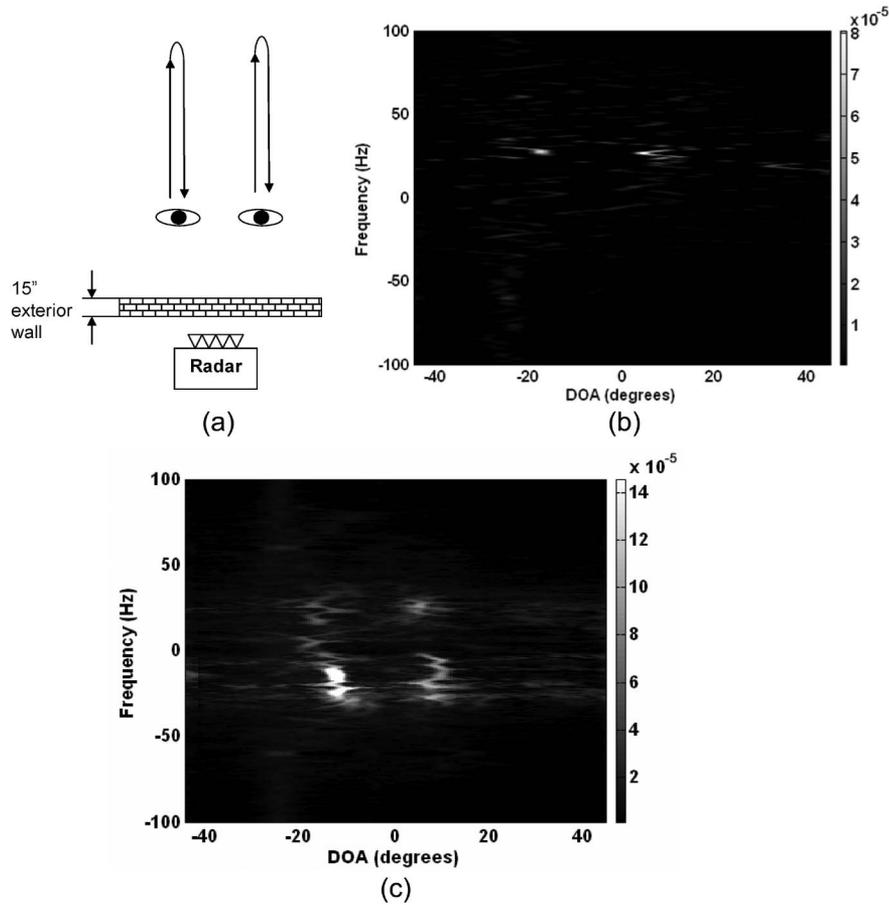
Fig. 5. Two human subjects in a through-wall scenario resolved in the DOA space. (a) Measurement setup. (b) CLEAN result for a single time instant. (c) Time-integrated CLEAN result.
