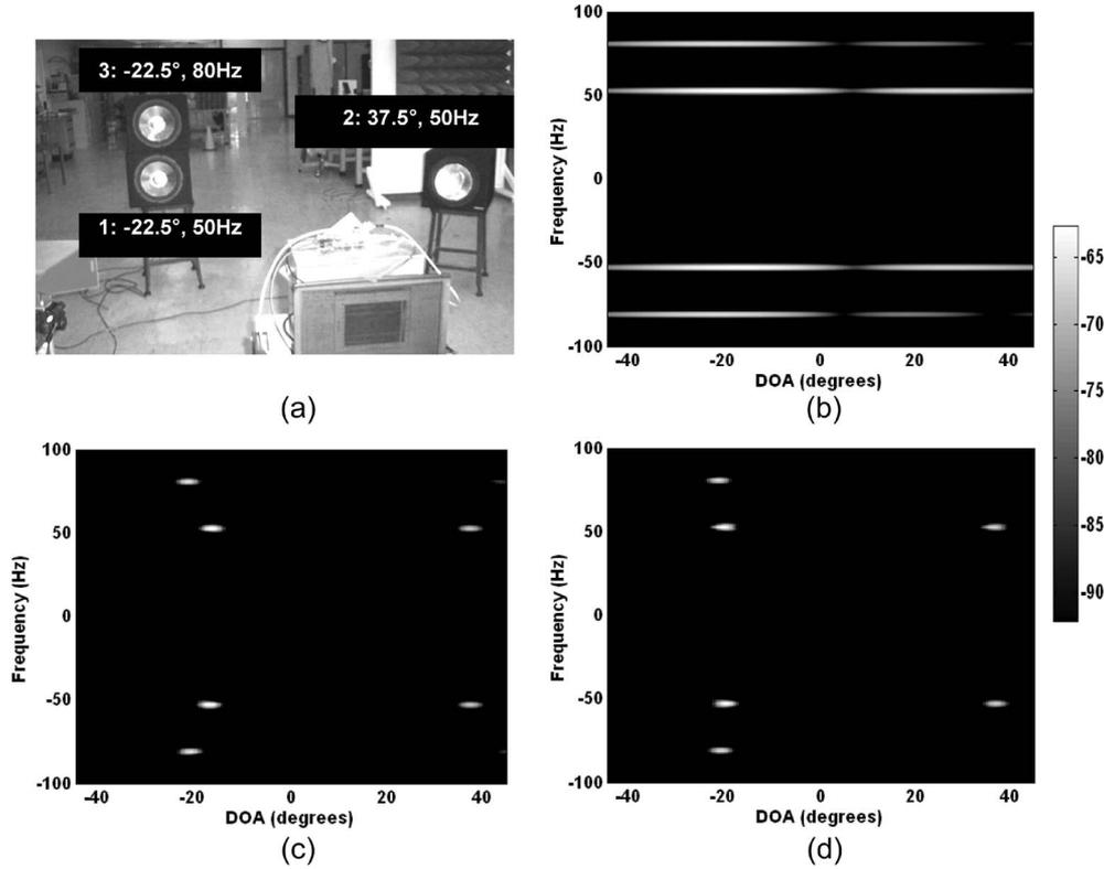
Fig. 2. Three loudspeaker targets in indoor LOS resolved in the Doppler–DOA space, in decibel scale. (a) Experimental setup. (b) Beamforming result. (c) CLEAN result. (d) RELAX result.
