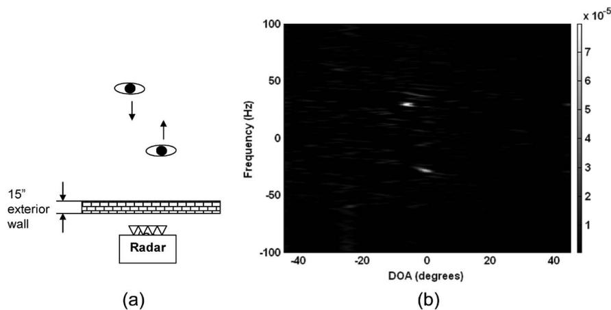
Fig. 4. Two human subjects in a through-wall scenario resolved in the Doppler space. (a) Measurement setup. (b) CLEAN result.
