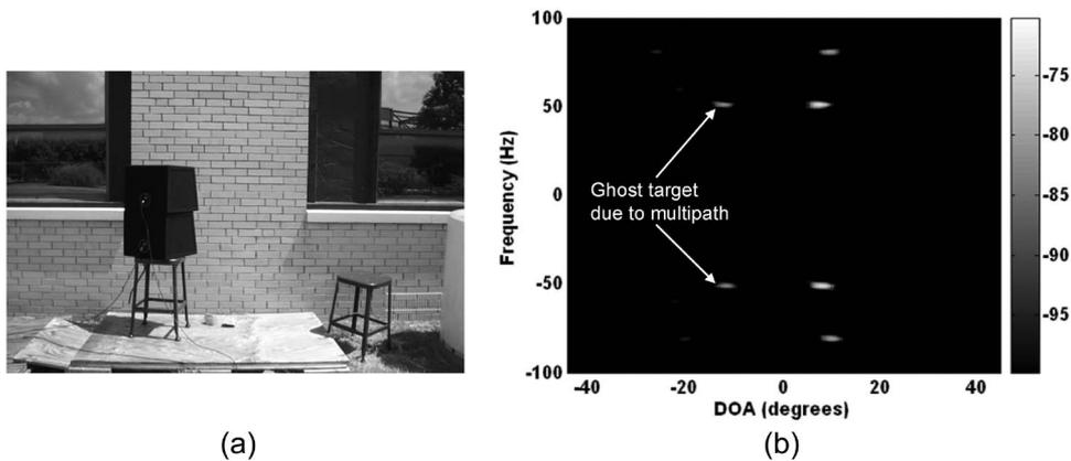
Fig. 6. Two loudspeaker targets in a through-wall scenario resolved in Doppler, in decibel scale. (a) Experimental setup. (b) CLEAN result.
