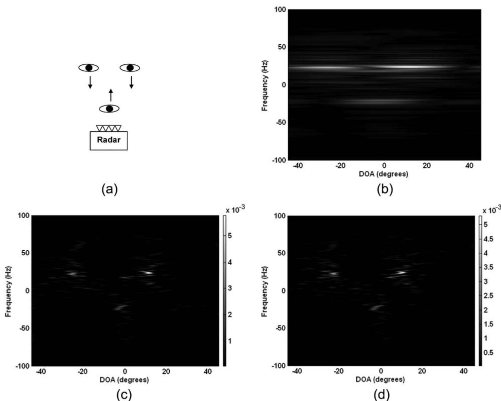
Fig. 3. Three human subjects in indoor LOS resolved in the Doppler-DOA space. (a) Measurement setup. (b) Beamforming result. (c) CLEAN result. (d) RELAX result.
