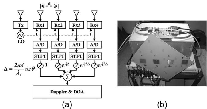
Fig. 1. (a) Radar architecture. (b) Photograph of the receiving array.
