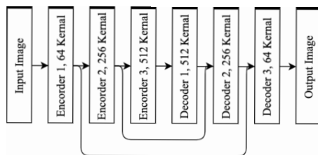
FIGURE 4. Simplified U-Net architecture for a generator network.
