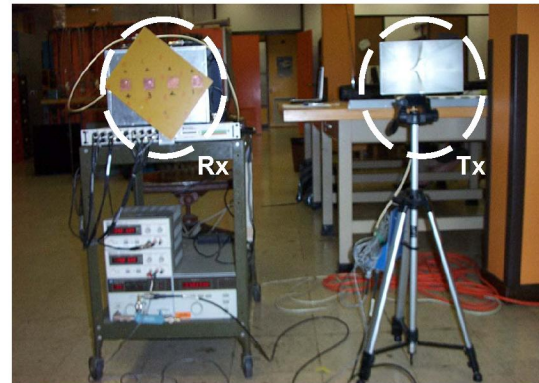
Fig. 4. RADAR set up
