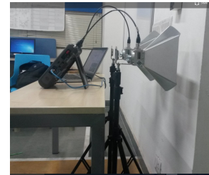
Fig. 2. Monostatic continuous wave through-wall radar configured using vector network analyzer and two horn antennas.
